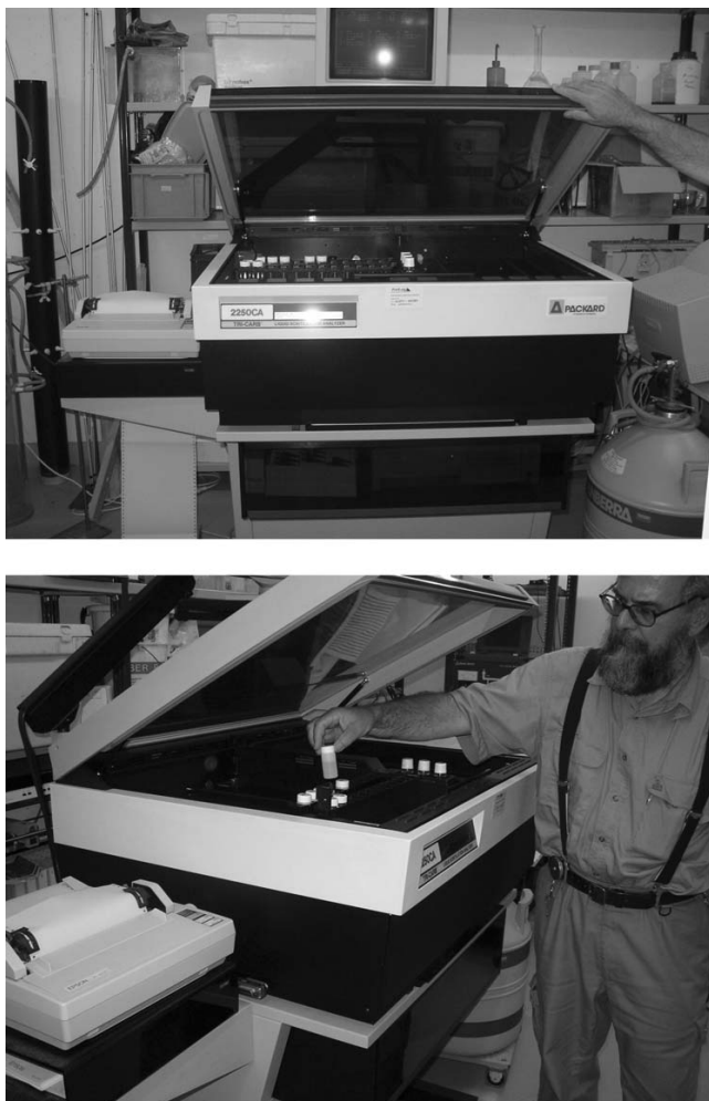
Figure 4.2. Liquid scintillation analyzer at the Centre of Hydrogeology, University of Neuchatel, Switzerland. The detection limit of this instrument is about 8 TU. Computer, shown in the top figure, is connected to the analyzer for processing the analyses. A sample vial is shown in the bottom figure.
